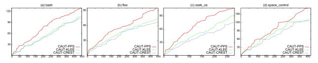
Fig. 5. MC/DC Coverage Testing, (a) bash (b) flex (c) osek\_os (d) space\_control, X-axis: iterations, Y-axis: covered decisions
