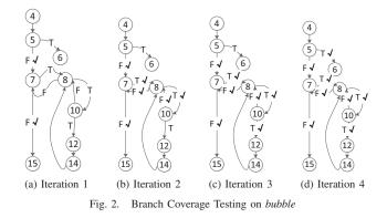
Here we denote a branch as the line number followed by T or F to respectively represent the true or false one. From the CFG, there are total 8 branches, i.e., 5F, 5T, 7F, 7T, 8F, 8T, 10F and 10T. In the following we illustrate the process under branch coverage testing. Suppose the initial input values of v and n are randomly initialized as [4, 0, 1, 8, 0, 2] and 0, respectively. After we test *bubble* within our framework, we could get the following test cases and corresponding execution paths:
